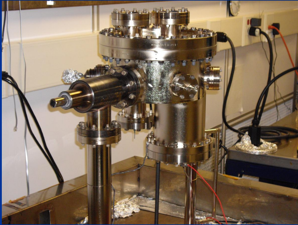
UHV detector/cathode processing station
