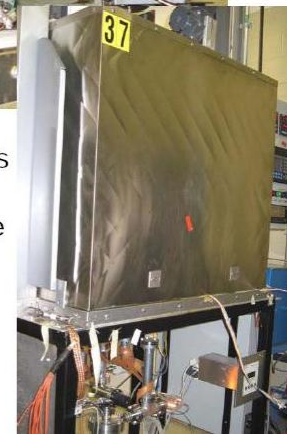
The oven cover was then lowered. The temperature was set to 150 C, which was the deposition temperature for the alkali metals.
