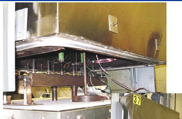
The oven cover was then lowered. The temperature was set to 150 C, which was the deposition temperature for the alkali metals.
