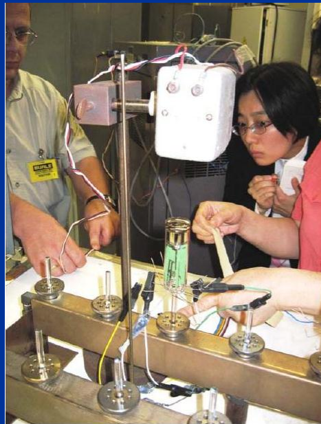
Making electrical contacts to the various electrodes. A "white" light source is also installed over the tube to monitor the photocurrent during deposition
