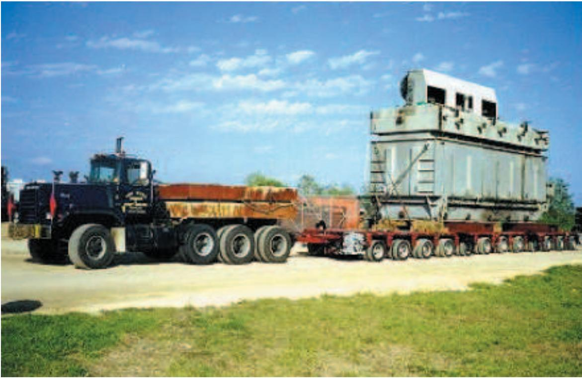
Figure 4: Goldhofer hydraulic platform trailer.
