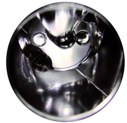
AFTER 12HRS OF EP 150 \mu m Nb REMOVED
