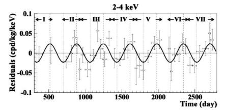
**Figure 8** The DAMA annual modulation signal, showing the variation in count rate from the average over a seven-year data-taking period in a 2–4 keV<sub>ee</sub> energy bin.
