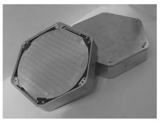
**Figure 9** Mounted CDMS II ZIP detectors (75 mm diameter) made of either Ge (250 g) or Si (100 g).
