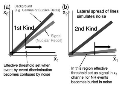
**Figure 11** The plots represent background and signal event distributions in discriminating detectors, which use the ratio of measured quantities  $x_1$  and  $x_2$  to characterize the event. The two kinds of threshold effects arising from the relative ratios of the discrimination parameters are shown in (a), where signal and background distributions become confused, and (b), where  $x_2$  falls into noise for signal events.
