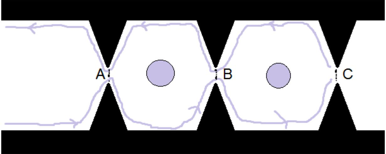
Figure 4: Diagram of device to measure and braid quasiparticles.
