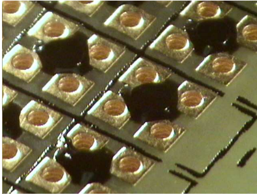
Figure 8: A test in which epoxy was deposited under machine control at the juncture of four of the Burle anode pads (in this case the mating board was glass, so we could see how we did [25]).
