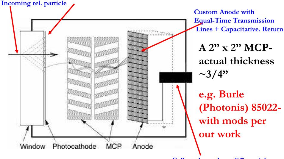
Collect charge here-differential Input to 200 GHz TDC chip
