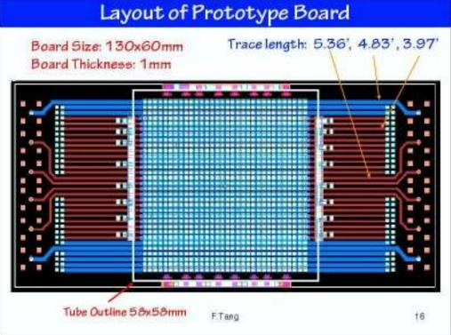
32 50 ohm transmission lines on 1.6 mm centers (Tang); attach to 1024 anode pads (Sellberg)
