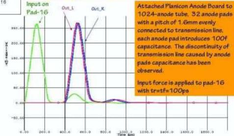
Simulation of loaded transmission line With mock MCP pulse and anode pads (Tang)
