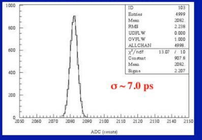
Two Burle/Photonis MCP-PMTs with 10 µm MCP holes operating at 2.85 & 2.43 kV. Ortec 9327Amp/CFD (two) with a walk th. of +5mV & TAC566 & 14 bit ADC11
