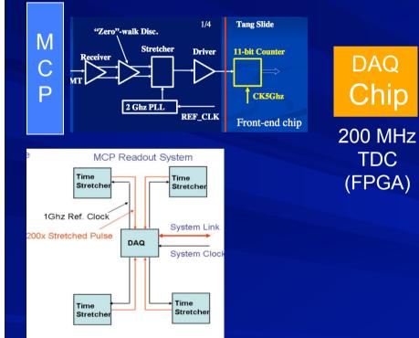
Fig. 2: The time stretcher receives signal from MCP, a very low timing jitter/walk discriminator will be implemented to generate a "start" signal. The time to measure is the difference between "start" and "Stop", that is a 500ps-1ns time interval pulse . With the following 1:200 time stretching circuit, a stretched pulse (100n-200ns) then be sent to DAQ chip for digitizing by a 11 bit counter with 200ps resolution.
