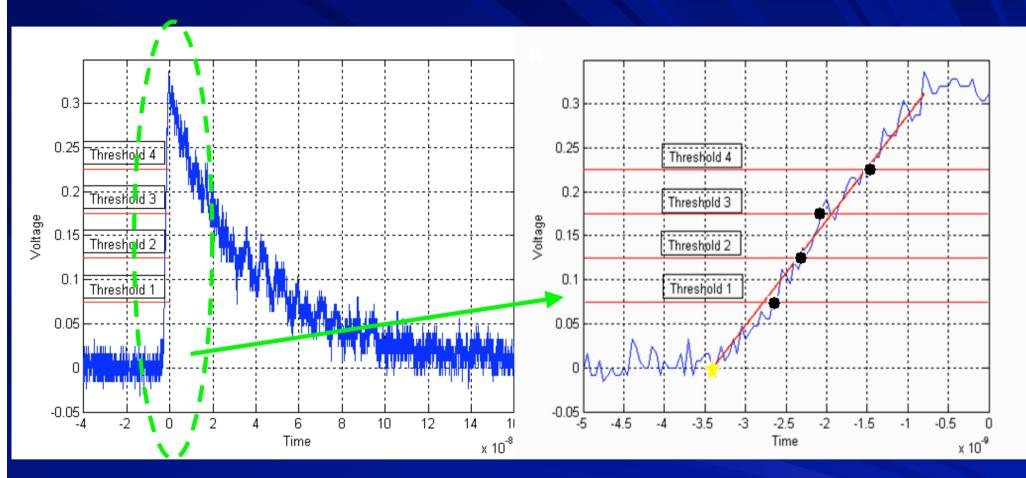
A sample pulse generated by LSO/PMT (50ps sampling interval)
