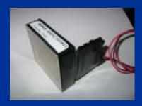
Photonis MCP-PMT 85012-501 (64 pixels, ground all pads except one)
