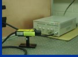
Hamamatsu PLP-10 Laser (Controller w/a laser diode head) 405 & 635nm head.
