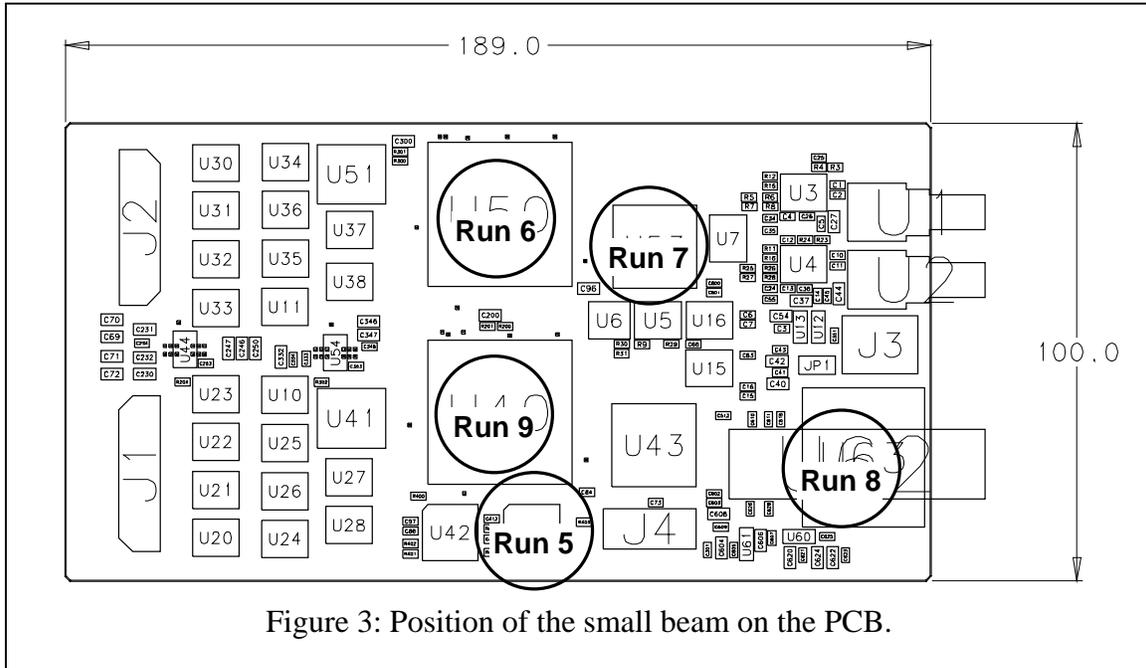
Figure 3: Position of the small beam on the PCB.
